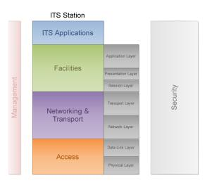
Fig. 1. The ETSI and OSI communication stacks [9].
