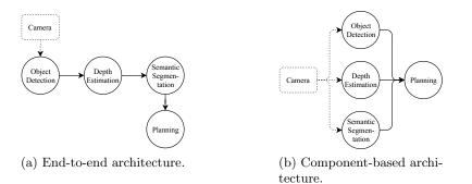
Fig. 1: Functional architectures for a scene understanding system in autonomous vehicles.
